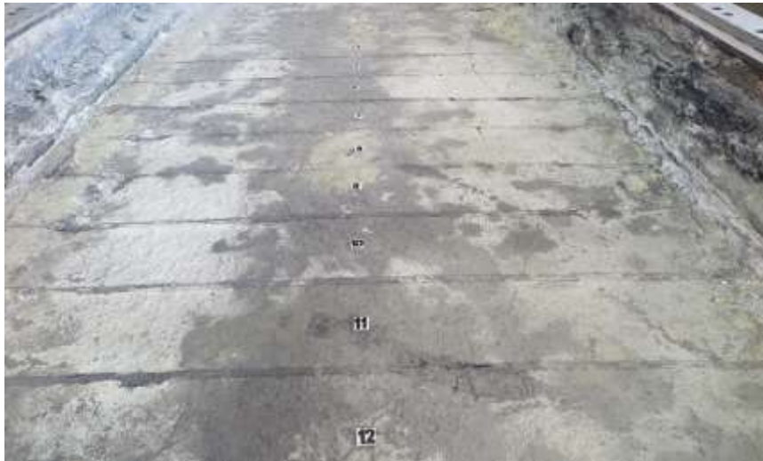
Figure 14. Cleaned DX pot cavity with CleO 2 paste at 369 days.
