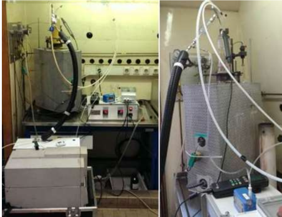
Figure 5. Equipment to follow-up PAH and VOC emissions during paste baking.
