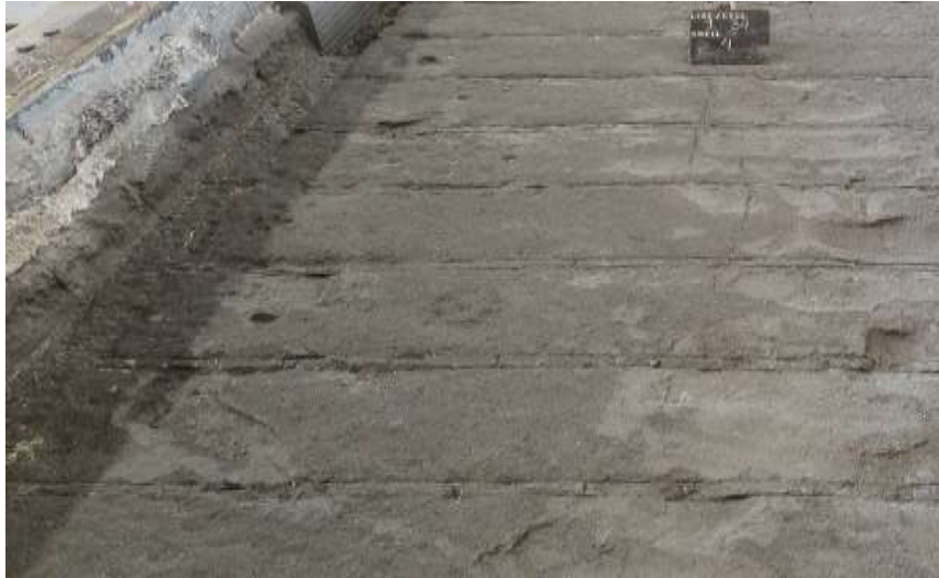
Figure 13. Cleaned D18 pot cavity with NeO 2 paste at 680 days.
